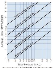
This chart is based on SMACNA HVAC Air Duct Leakage Test Manual, 1985 Edition found in Figure 4-1 under "Duct Leakage Classification".
